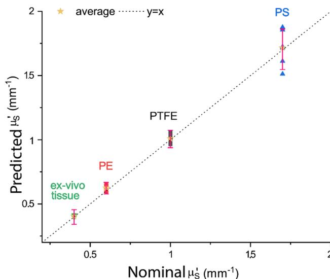
**Figure 3.** Plot of the predicted reduced scattering coefficients vs nominal values of four turbid samples using SORS. The yellow stars indicate the average value predicted from all spatial offsets. The system was calibrated on the PTFE values (black filled squares). Error bars (magenta) denote the average error of prediction.
