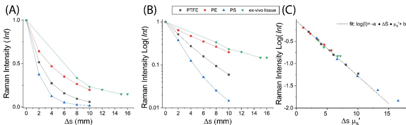
**Figure 2.** Raman intensity decays vs SORS spatial offset measured for the four model samples: (a) linear plot normalized to zero offset value and (b) log plot. (c) Log plot of the Raman intensity vs unitless  $\Delta s \mu_s'$ . Linear fit (black dotted line) of the PTFE data (black filled squares) show the calibration model used for the prediction of  $\mu_s'$ .
