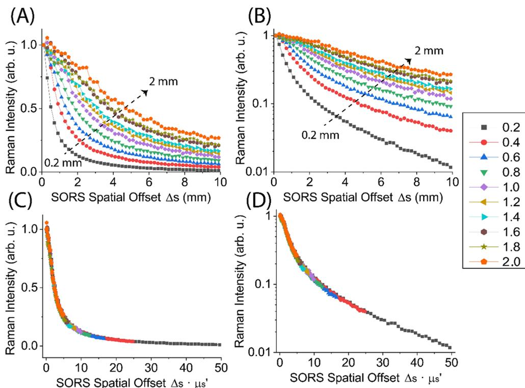
**Figure 1.** Raman intensity decay for point-like illumination and collection SORS geometry as a function of the SORS spatial offset ( $\Delta s$ ) derived from Monte Carlo simulations shown in (a) linear and (b) logarithmic scales. The same data normalized to unitless spatial offset expressed as the product of SORS spatial offset and  $\mu_s'$  shown in (c) linear and (d) logarithmic scales. The legend on the right applies to all the plots and indicates medium transport lengths in mm's.
