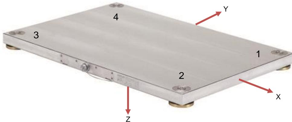
**Figure 17 Kistler force platform with four force sensors, and the directional axes of measurement**
