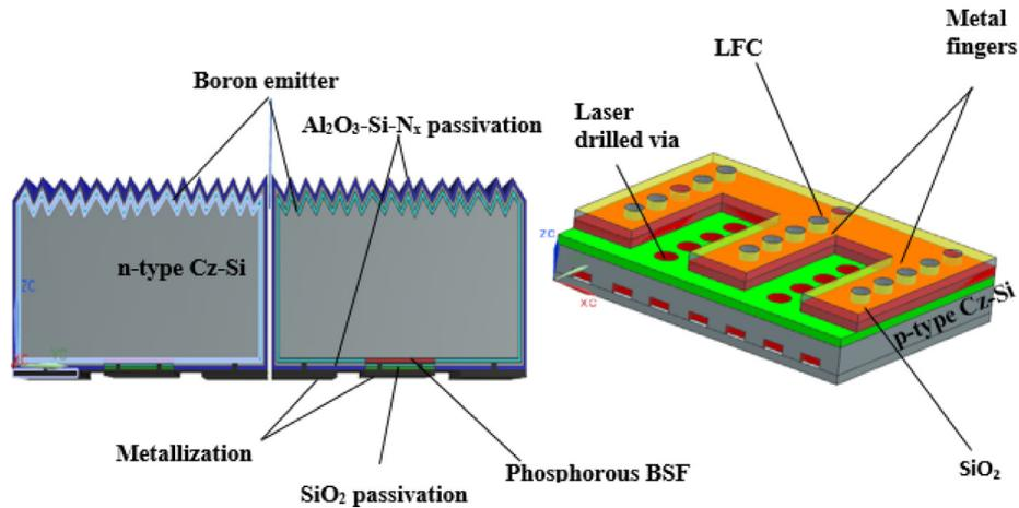
Fig. 8. Schematic cross section of the EWT solar cell.
