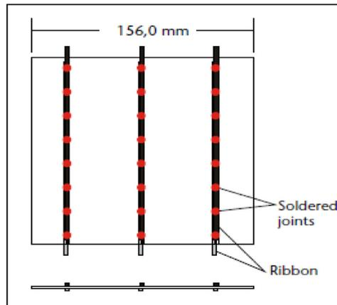
Fig. 5. Selective laser soldering of a 3-busbar solar cell [143].
