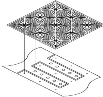
Fig. 13. Interconnection for a PUM one cell laminate.
