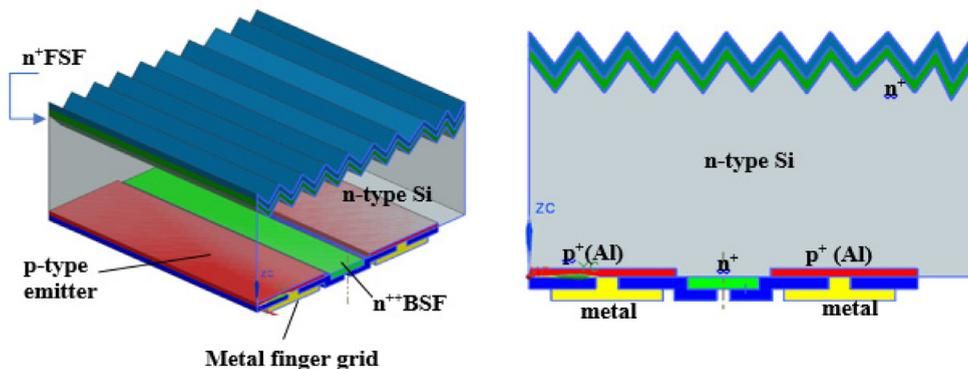
Fig. 10. Schematic n-type BJ-BC silicon solar cell.
