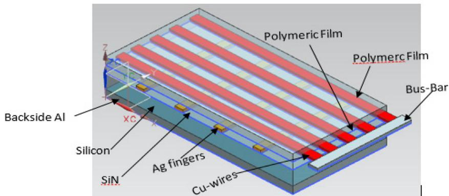
Fig. 18. Schematic of Day 4 Electrode.
