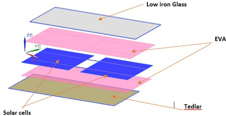
Fig. 4. Exploded view of a typical solar PV-module.
