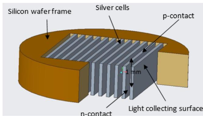
Fig. 15. Schematic drawing of Silver cells.
