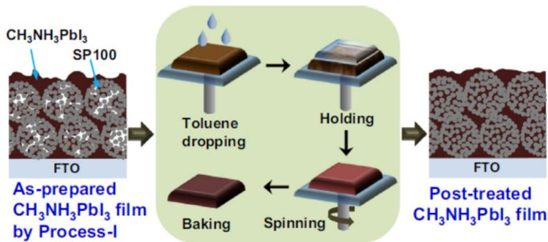
Fig. 17. SP100 Fabrication Process [144].
