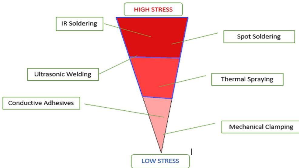
Fig. 19. Ranking of possible interconnection techniques in terms of induced mechanical stress.
