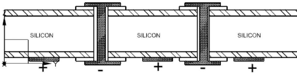
Fig. 12. Schematic of Pin-UP module cell interconnection.
