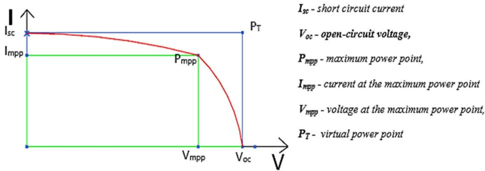
Fig 20. shows a schematic I-V curve of an illuminated PV module.
