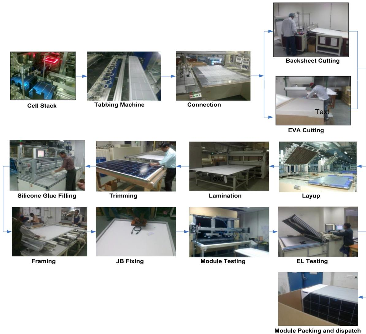
**Fig. 1.** The assembly process flow of c-Si PV-module.
