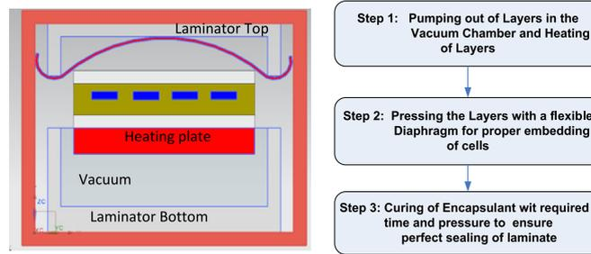
Fig 2. c-Si PV module lamination process.
