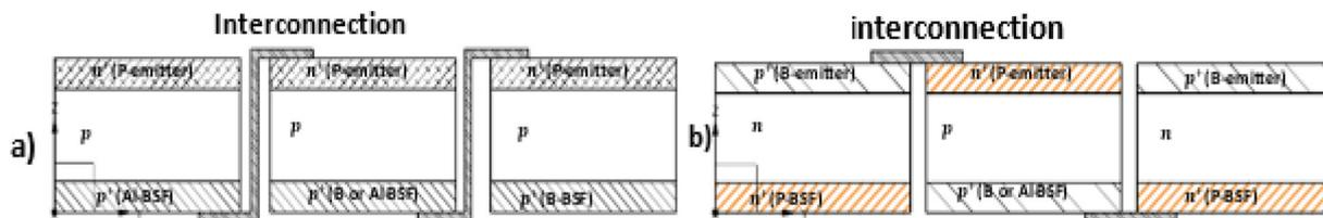
Fig. 11. (a) Conventional module interconnection: each cell backside is connected with the front side of the subsequent solar cell (b) Innovative interconnection using alternating p-type and n-type solar cells [16].
