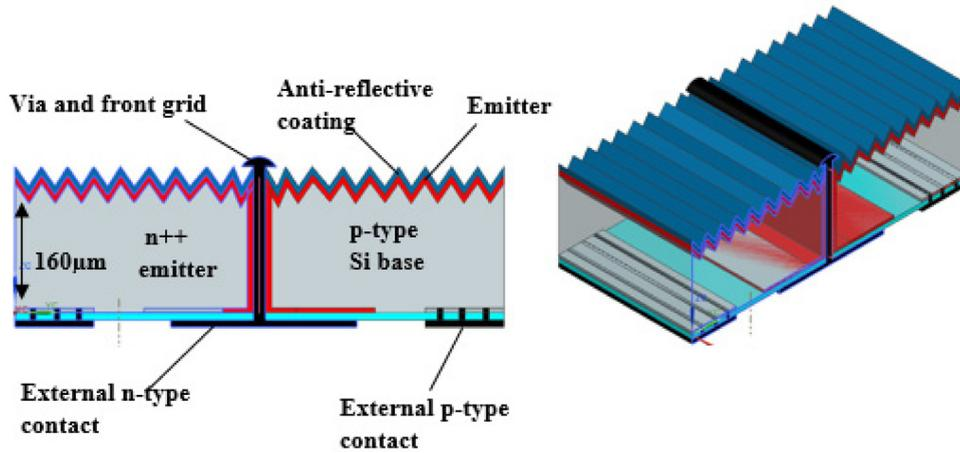
Fig. 9. MWT cell interconnection.
