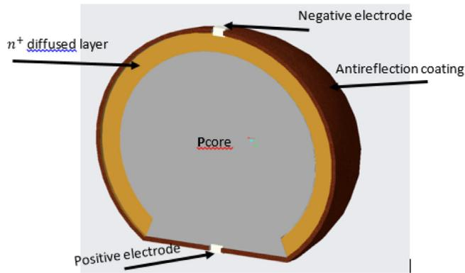
Fig. 16. Schematic of Spherical cell.
