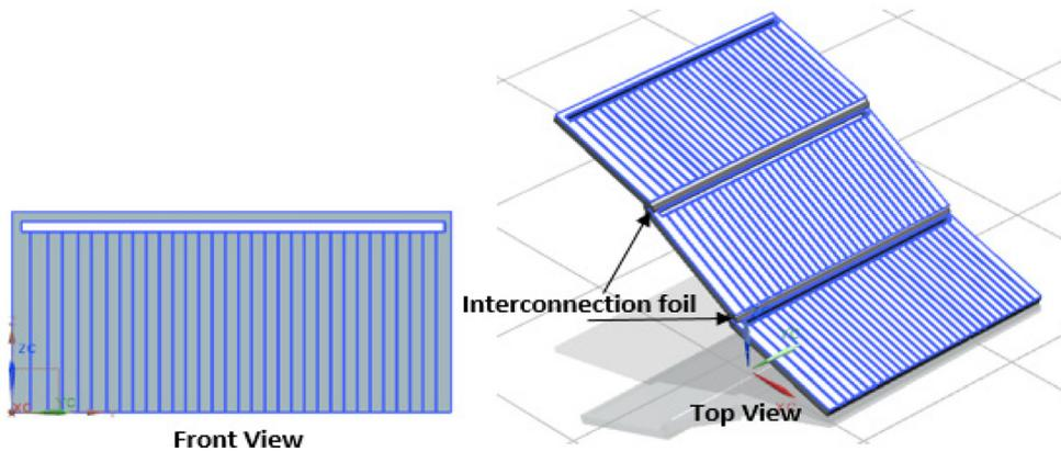
Fig. 7. Schematic drawing of a cell for shingled cells interconnection.
