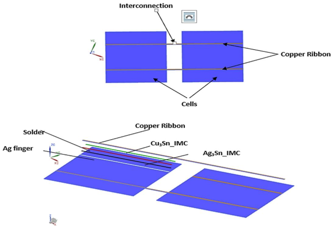
Fig. 6. Conventional front-to-back cell interconnection technology.
