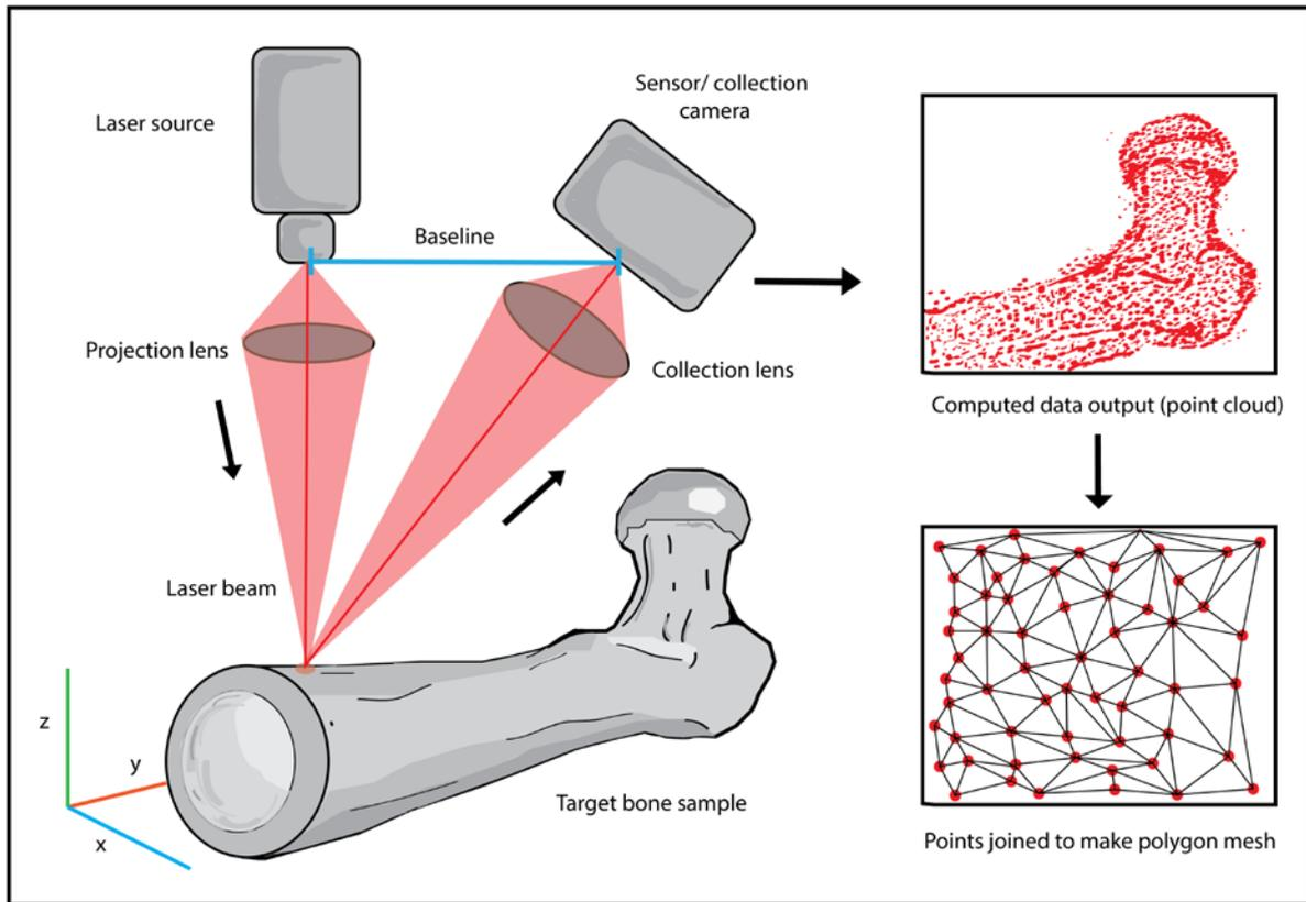
Figure 1: The recording method using a laser scanner
