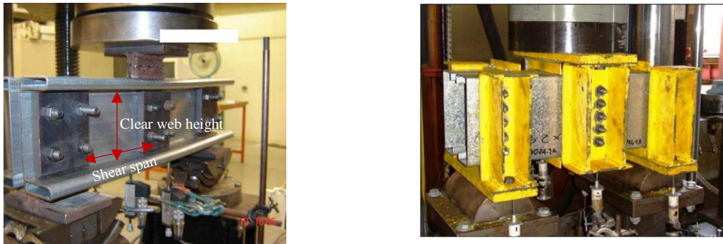
(a) Shear test set-up for hollow flange sections [21] (b) Shear test set-up for lipped channel sections [22]
