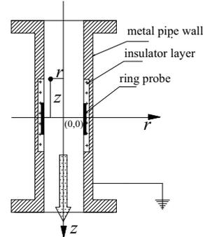
Fig. 2. Sectional View of ring-shaped electrostatic Sensor
