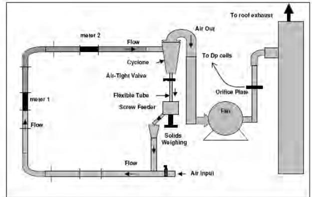
Fig.1. Pneumatic conveyor at the University of Teesside
