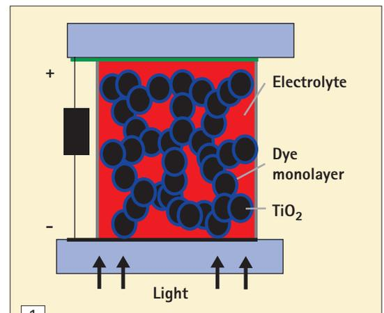
1 Schematic diagram of cell design for high efficiency dye sensitised solar cell (not to scale)
