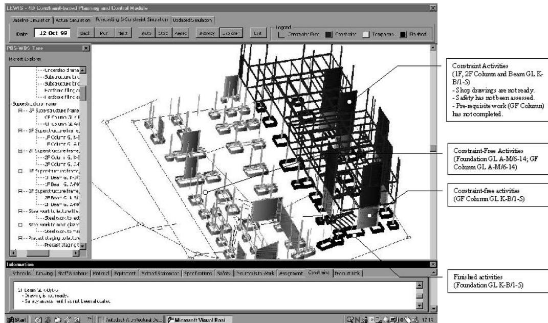
Figure-2: 4D Constraint-based Planning and Control Prototype System
