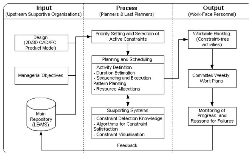
Figure-1: 4D Constraint-based Planning and Control Framework
