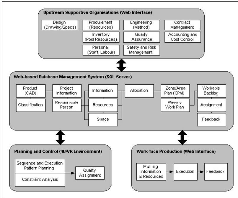
Figure-2: LEWIS System Architecture
