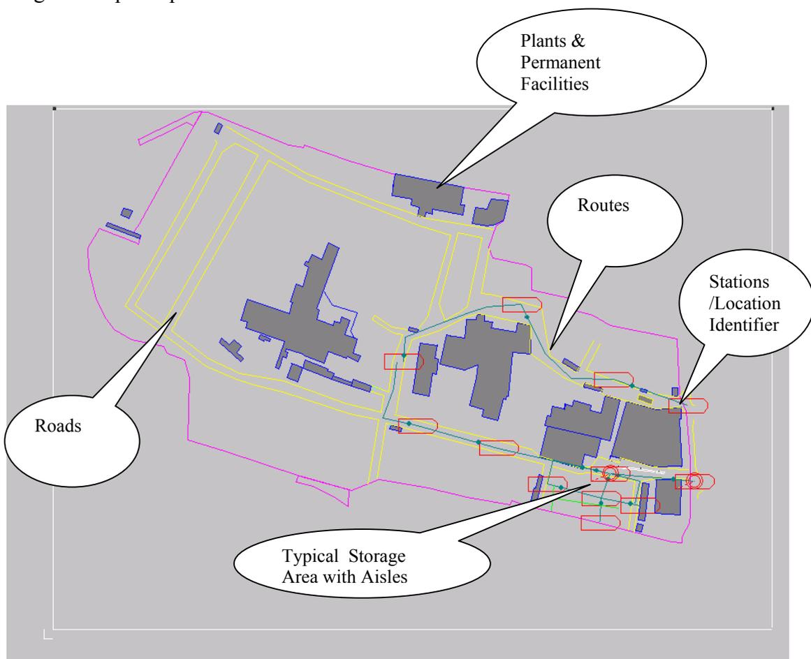
Figure 5: Sample layout and modelling of stockyard operations in ARENA
