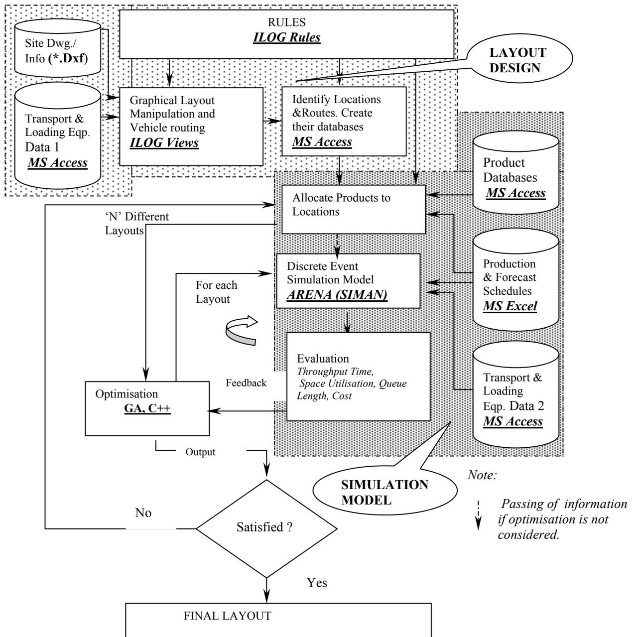
Figure 2. Simulation model and its integration with other components of Stockyard Layout Management Model
