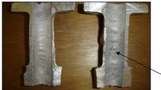
**Figure 28. Core blow defect on the sectioned Al-LM25 (core removed)**
