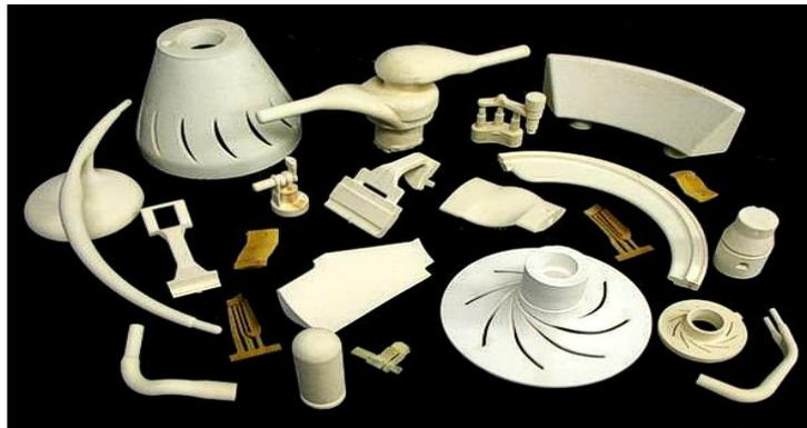
**Figure 2. Examples of different ceramic core shapes** <sup>(10)</sup>
