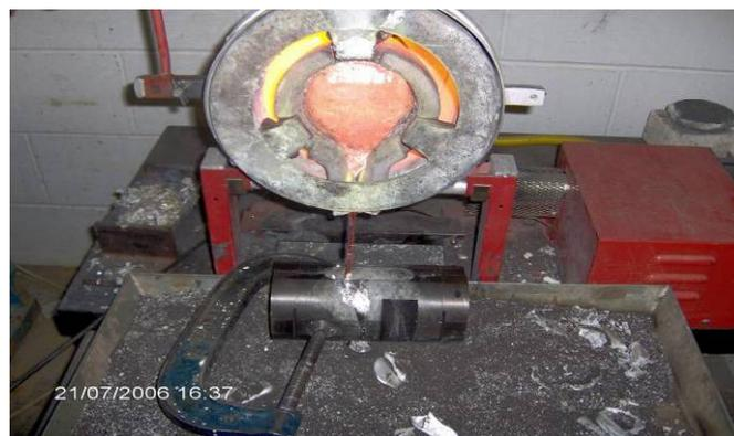
**Figure 13. Pouring process to assembled mould**
