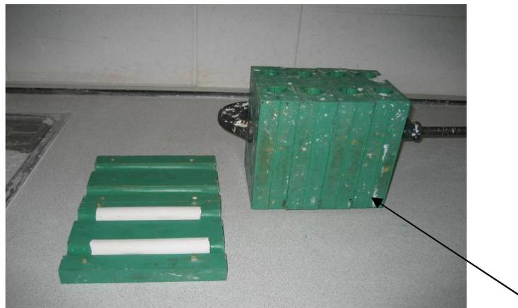
**Figure 29. Vertical standing wooden core boxes with cores**
