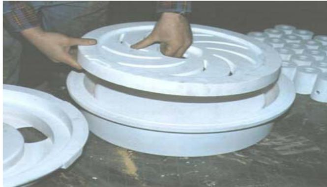
**Figure 4. Core being inserted into drag after curing<sup>(11)</sup>**
