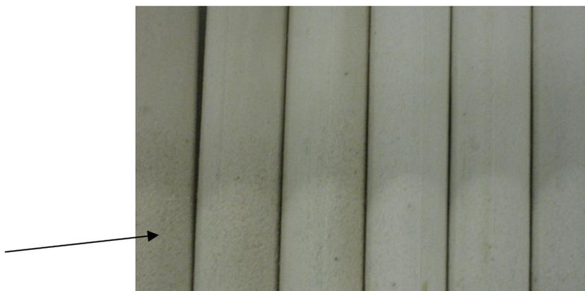
**Figure 30. Cores fired at 600 °C with the 30/50 fused silica settled in the bottom.**
