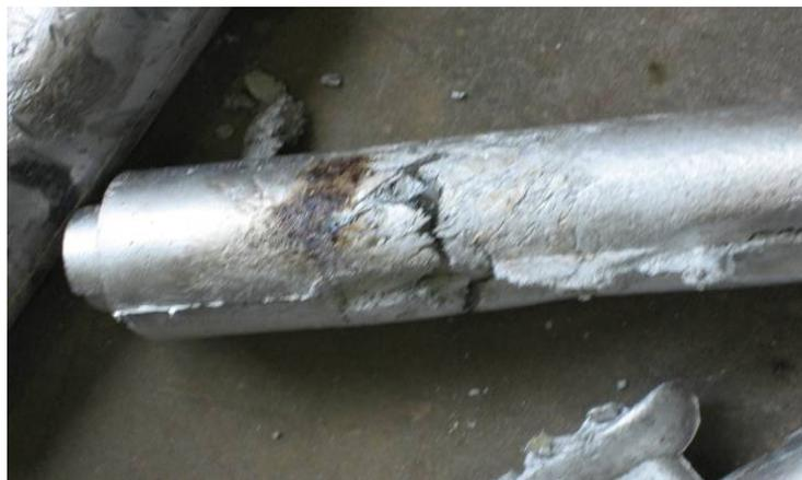
**Figure 41. Al-LM25 break since not feeding the metal properly**
