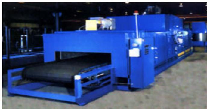
**Figure 5. Conveyor core drying furnace** <sup>(13)</sup>
