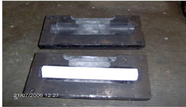
**Figure 12. Cast iron split moulds with core**
