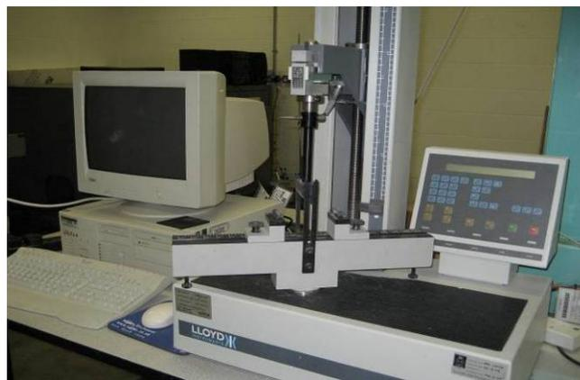
**Figure 10. LLOYD Universal test machine**
