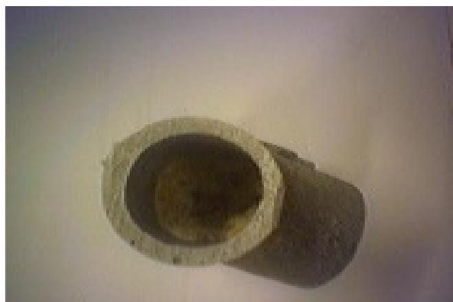
**Figure 26. Effect of diluted nitric acid on Trial 1E core fired at 400 °C under four hours.**
